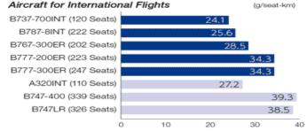
Note: Calculated for international flights (assuming flight distances of 5,556km for the B737-700INT and A320INT and 9,260km for all other aircraft types, with full seating) Retired aircraft (g/seat-km)
